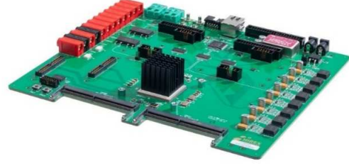
Fig. 2 SEE test board STB033A for DDR4 SDRAM memories
